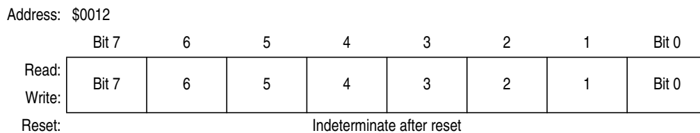
Figure 8-13. TIM Channel 0 Register Low (TCH0L)
